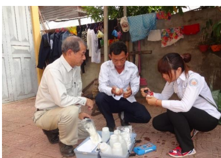
Residual chlorine measurement at tap in town every two weeks is continued after OJT in phase 2 (the left is the writer)
