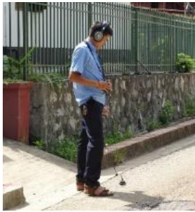
Photo 2: Detecting leak sound transmitted from buried pipe to the surface.
